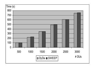
Figure 9: SWEEP vs. DyDa on Data Update Processing
