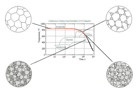
Fig. 7. CCT Diagram and Predicted Microstructures
