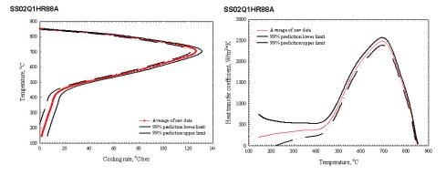
Fig. 10. Cooling Rate Curve
